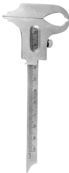
Fig.2 HI-08-194 Boley Measuring range 0-100 mm
